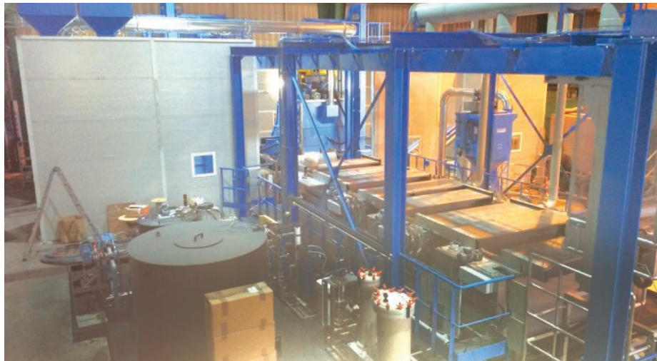
Polymer coating is a four-step automated process that can be directly incorporated to a forging line.
